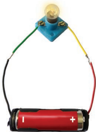
Fig. 3.9: An electrical circuit
