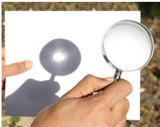
Fig. 5.7(a): Focusing the sunrays using a magnifying glass
