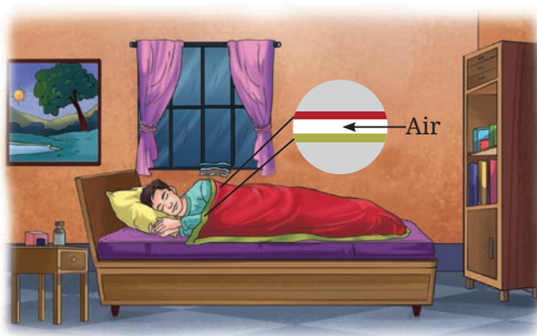
Fig. 7.2: Air trapped between two thin blankets acts as an insulator
