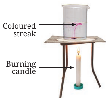
Fig. 7.5(b): Demonstration of convection in heated water
