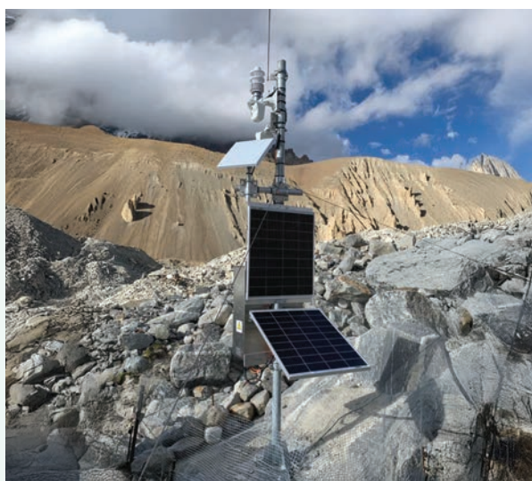
Fig. 2.12. AWS at a glacial lake of Sikkim
